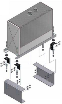
Pre-Packaged Kit Includes: Steel or aluminum tank assembly with (2) 1 ¼" screw-in NPT bottom ports, filler/breather assembly including a 40-micron filtered breather cap (chain-mounted), auxiliary vent and an ASK-200 mounting kit.
