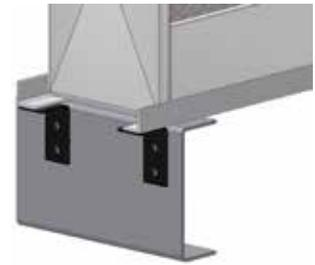
**Note: The top of the mounting angle should be flush with the top of the chassis rail.**
